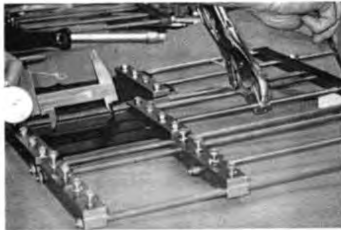
(a) Method of applying tensile load to test specimens in Part III tests
