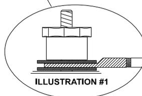
\* REMOVE CT JUMPERS FROM SECONDARY TERMINALS AFTER WIRING TO TEST SWITCH AND METERS HAVE BEEN APPROVED BY PRIMARY SERVICES
