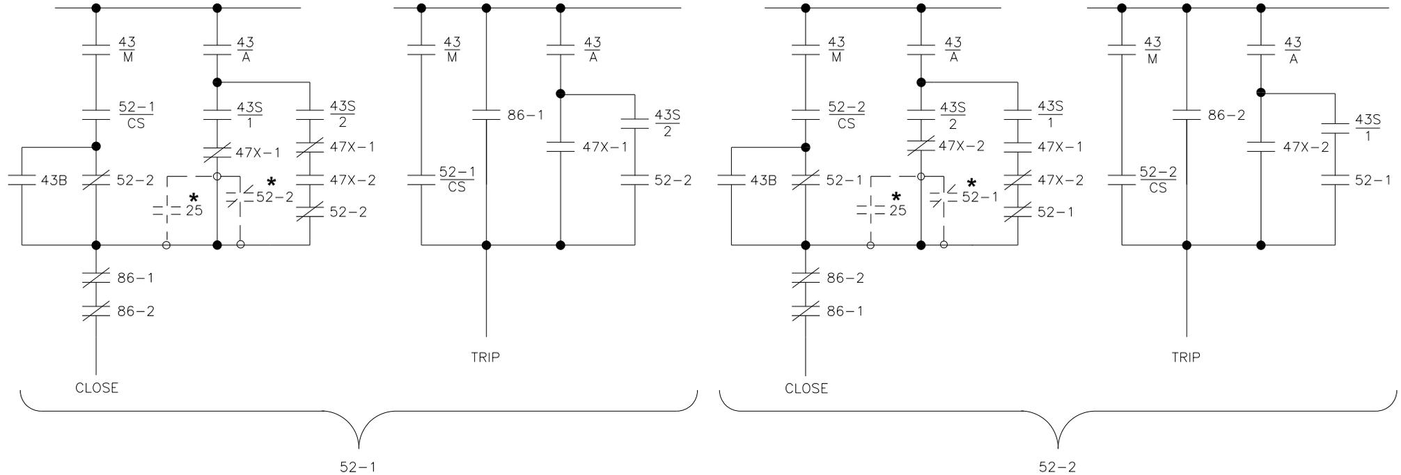
PARTIAL SCHEMATIC – ATO SCHEME (NORMAL-ALTERNATE) W/ NORMAL LINE SELECTION
