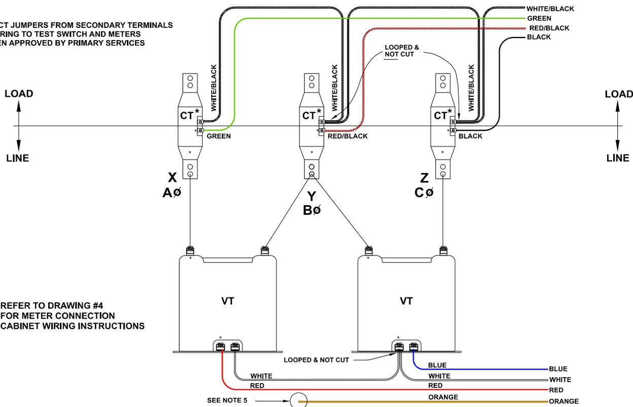
REFER TO DRAWING #4 FOR METER CONNECTION CABINET WIRING INSTRUCTIONS
