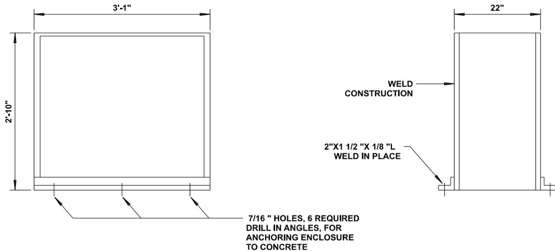
**ENCLOSURE TO BE CONSTRUCTED OF 11-GA SHEET STEEL**
