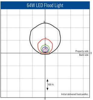
Distribution: 6 H x 6 V NEMA Initial delivered lumens: 9,600 Luminaire mounting height: 26 feet Aiming angle: 60° from horizontal
