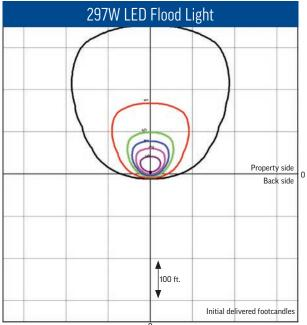
Distribution: 6 H x 6 V NEMA Initial delivered lumens: 37,400 Luminaire mounting height: 26 feet Aiming angle: 60° from horizontal
